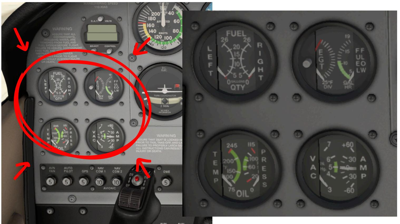
**Oil Pressure:** the force from the oil pump pushing oil through the engine to lubricate, cool, and clean moving parts, preventing metal-on-metal contact
