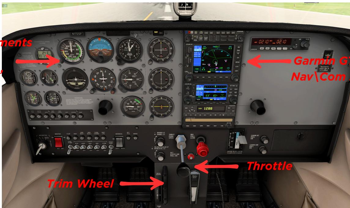
**Pitot Heat Switch:** an electric heating element that keeps the pitot tube from icing over, which would cause the airspeed indicator to malfunction (also acts as a stall warning sensor!)
